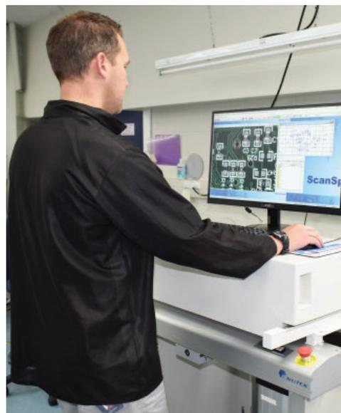
Haydon can inspect the PCA, soldering and component marking to very high magnifications.
